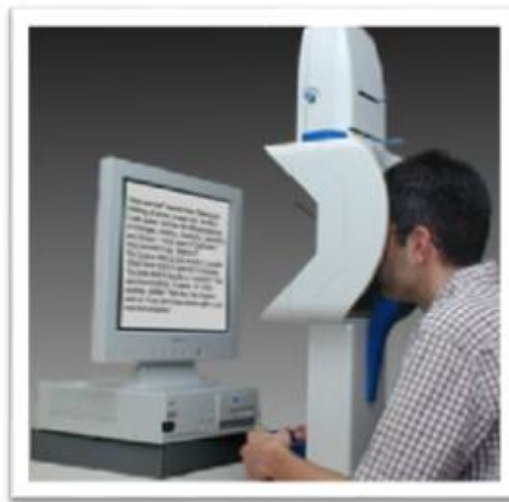
Figure 2.6: SMI hi-speed TM-ET sampling rate of 1250 Hz [27]
